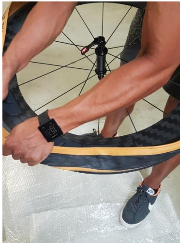
Pic 5, tire over the rim (you may want to use/support your work with tire levers)
